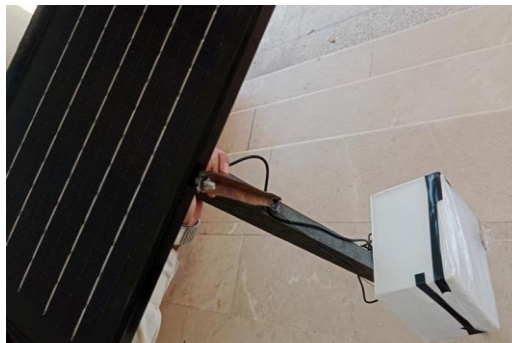
Figure 2. IoT-based sensor module developed for mango orchard.
