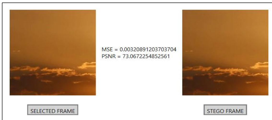
Figure 6. Comparison of MSE and PSNR for original and stego frames [720 x 480] confirming visual quality retention.
