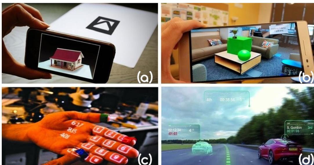
**Figure 2. (a).** Marker-based AR, **(b).** Location-based AR, **(c).** Projection-based AR, **(d).** Superimposition-based AR. [18]
