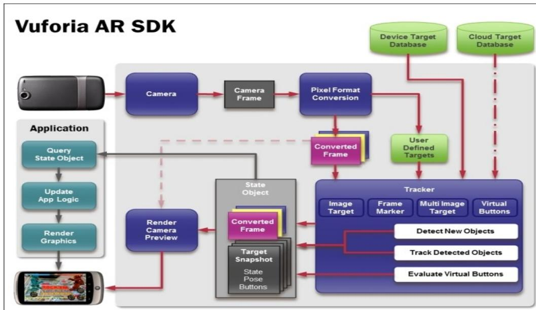
Figure 4. Flow diagram of Vuforia SDK [19]
