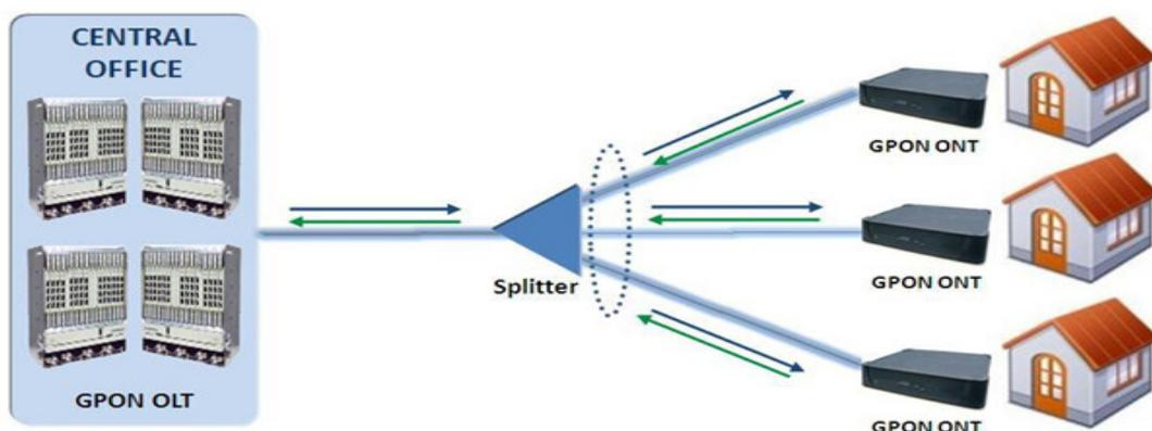
Figure 1. GPON networking with splitter
