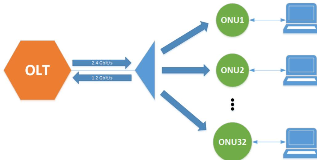
**Figure 2.** P2MP Topology configuration
